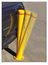
An internally welded, steel spring allows the bollard to flex on impact, absorbing the force of a collision and minimising damage to the bollard. Fewer damaged bollards means a cost saving on replacements. These bollards are ideal in high traffic areas.
